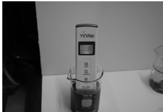
adjusting ph to 3 with dilute acid solution HCL
